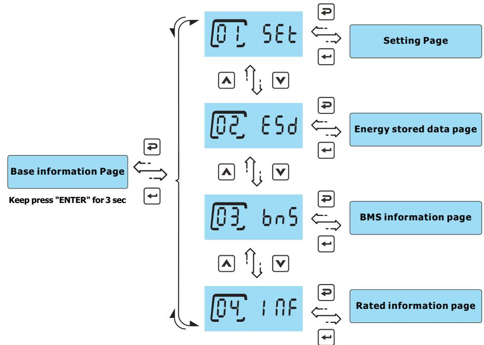
On base information page, pressing and holding "ENTER" key for 3 sec, the unit will enter parameters page. Press "UP" or "DOWN" key to switch the selection and press "ENTER" key to enter selected page. Press "ESC" key to back to previous page.
