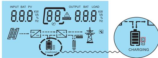
5. Roll LCD real time information pages by pressing "UP" or "DOWN" button, as below page, you can see the parameters of SOC and battery pack units in the communication system.
