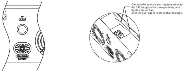
3. Make sure the wires are securely connected.
