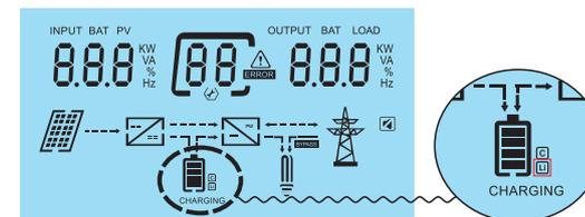
4. Power up lithium battery and inverter. Wait a moment, if the communication is built between them, LCD will show you "C" icon as below.
